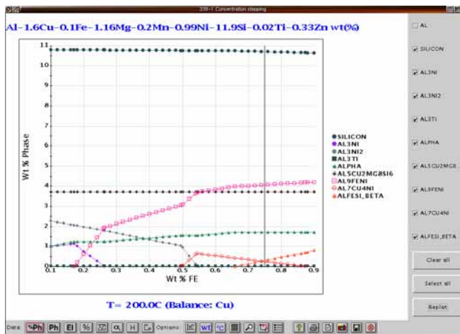
Concentration stepping: example of Al alloy 339-1
